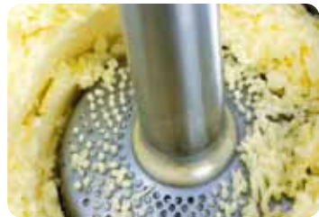
Stainless steel perforated grid and blade can be easily dismantled for cleaning.
